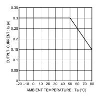
Fig.4 Derating curve
