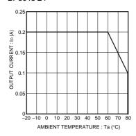
Fig.12 Derating curve
