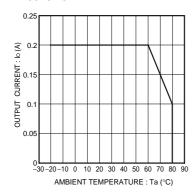
Fig.8 Derating curve
