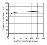
Fig.7 Conversion efficiency
