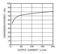
Fig.15 Conversion efficiency
