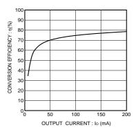
Fig.11 Conversion efficiency
