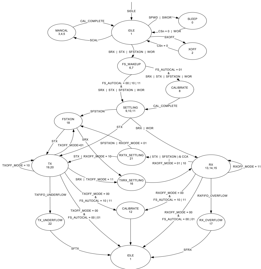
Figure 16: Complete Radio Control State Diagram
