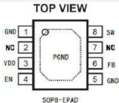
**Figure 3. PIN Configuration**
