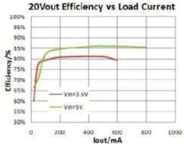
**Note:** Efficiency data is based on demo test at 20°C . If work at big current for long time, maybe thermal shutdown. its load capacity is related with heat dissipation conditions.
