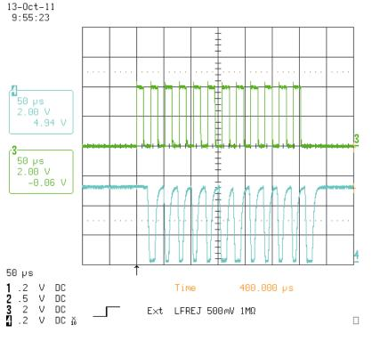
Green waveform: optical input signal to the photodiode that is connected to the amplifier circuit.
