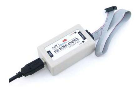
Debugger and programmer for C8051Fxxx MCUs, USB connection to the PC, JTAG and C2 debug interfaces to the target board
