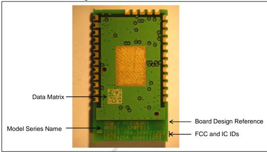
Figure 5. Bottom view of the module
