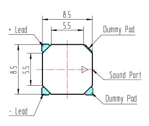
\*Unit: mm; Tolerance: ± 0.3mm Except Specified
