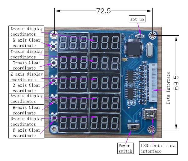
This product comes standard with HY-TB5DV-M driver board, using the appropriate cable docking HY-TB5DV-M driver board corresponding to digital interface, digital products obtained directly from the drive plate into the 5V power supply, no external power supply is
