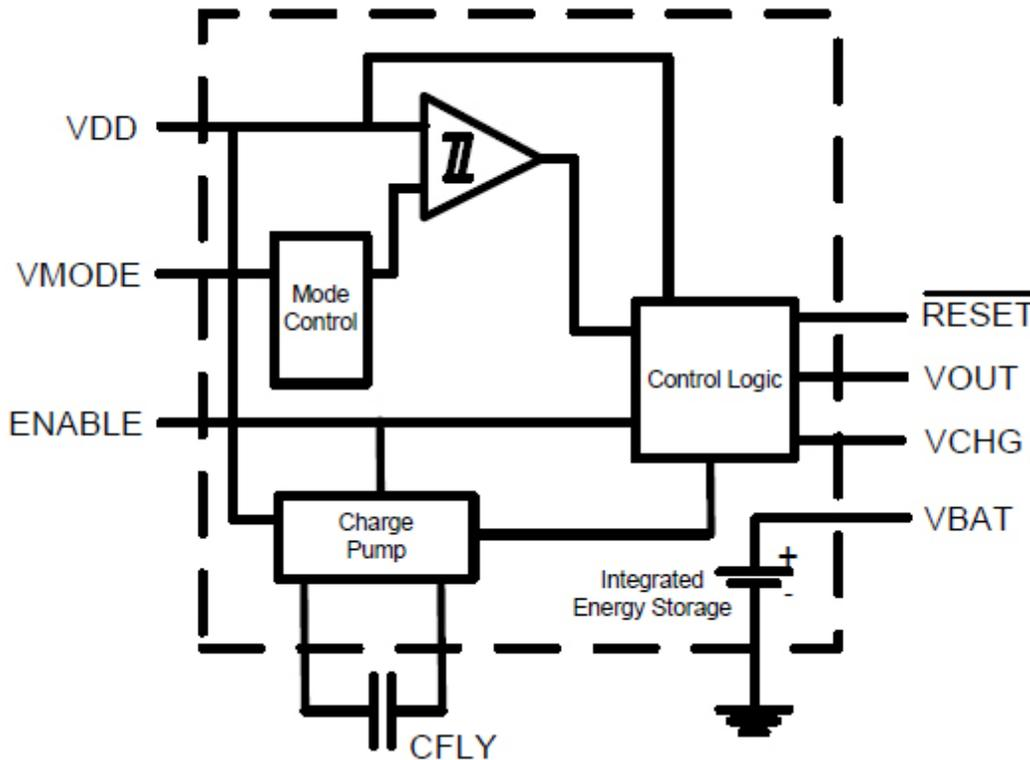
Figure 2: EnerChip CC CBC3112 Internal Block Diagram
