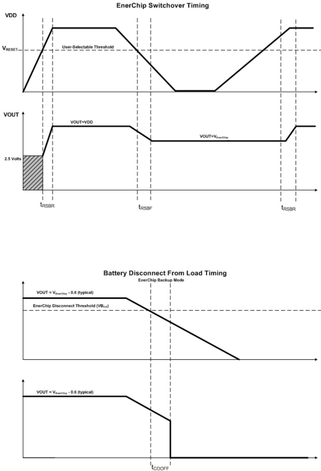
**Figure 4: EnerChip CC Switchover and Disconnect Timing Diagrams**
