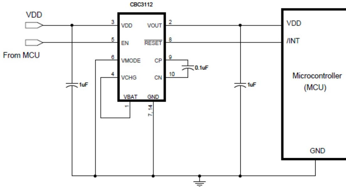
**Figure 6: CBC3112 Typical Circuit for Mode 1 Operation**
