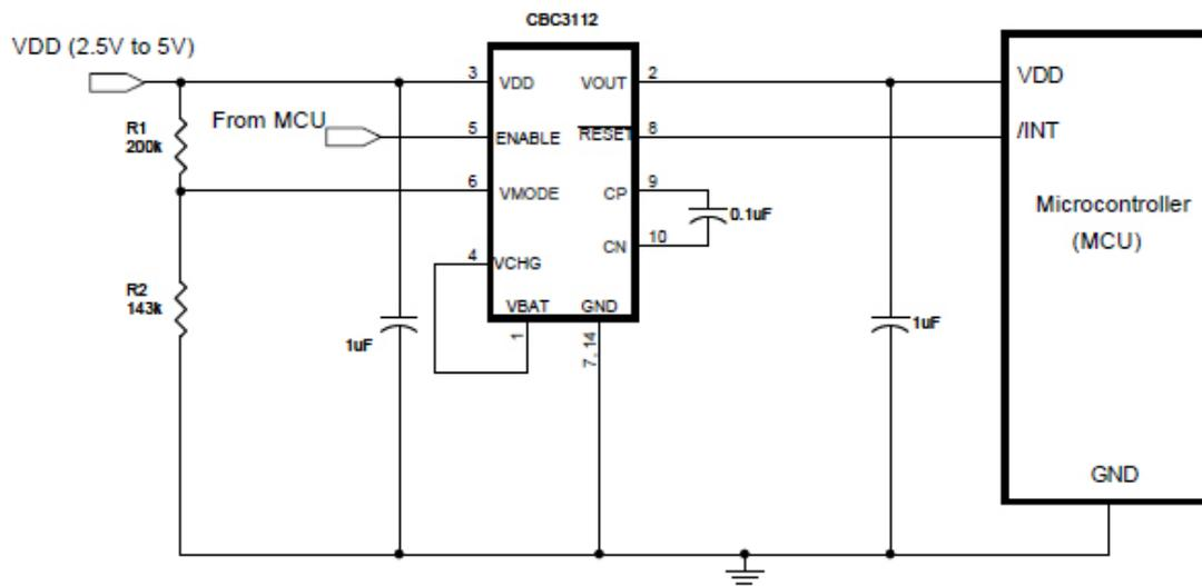
**Figure 7: CBC3112 Typical Circuit for Mode 2 Operation**
