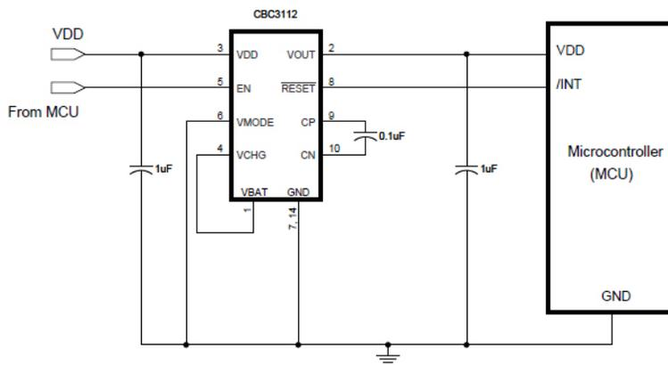
**Figure 1 - Typical EnerChip CC Application Circuit**
