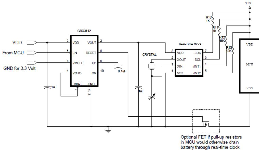
Figure 10: EnerChip CC Providing Real-Time Clock Backup Power
