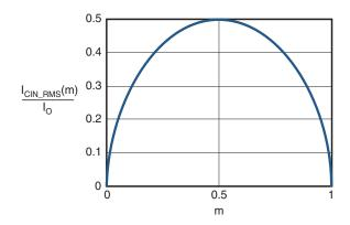
Figure 4. I<sub>CIN</sub> vs. Voltage Conversion Ratio
