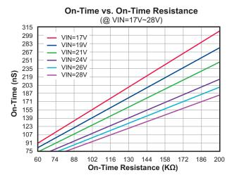
Figure 3. T<sub>ON</sub> vs. R<sub>TON</sub> Curves for AOZ2262AQI-18
