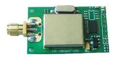
YS-1100 series is high data rate module for Serial data to RF. It bases on high performance RF IC and MCU, works on 433Mhz ISM frequency band, half duplex integrated receiving and transmitting. Modules could directly connect with monolithic processors, PC, RS485 devices, and other UART components with RS-232, RS-485 and UART/TTL level interface port. Transparent data interface, nakedness, and wide temperature design handles most industrial application though indoor/outdoor environments.
