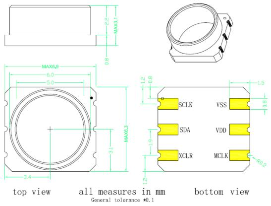
HP03 Series of calibrated sensor module HP03MA
