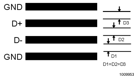
FIGURE 9. Recommended Diode Trace Layout
